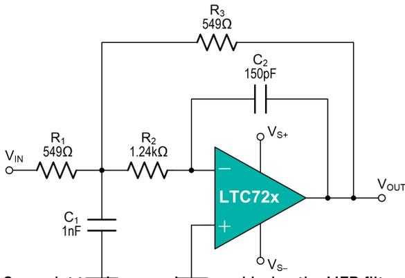
One point to observe when considering the MFB filter is that the output is inverted, relative to the input. If this inversion is not required, or not desired, a non-inverting output can be achieved through one of these options:
