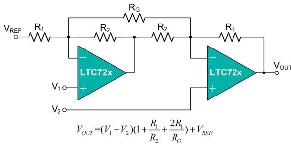
Figure 9. Instrumentation Amplifier
