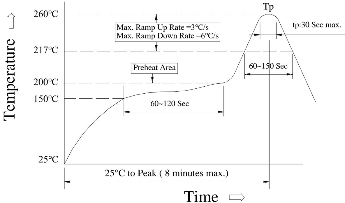
(1) Reflow Soldering Method :
