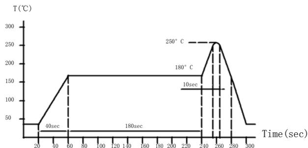
The reflow condition recommended above is according to the machine used by our company. Big differences will arise as a result of the type of machine, reflow conditions, method, etc used. Hence, before setting up your reflow conditions, please confirm with the above./上面推荐的回流焊试验条件是根据本公司的回流焊设备测试结果得到.不同的试验设备、试验条件和试验方法及试验结果不同.因此回流焊试验条件的设定需要仔细地确认.
