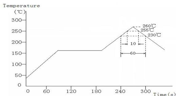
No mechanical and electrical defects are found after testing based on the above profile and keeping under the conditions of room temperature and humidity for 2 hours./在该条件下进行回流焊,常温常湿条件下放置 2 个小时后,无机械,电气特性缺陷发生.
