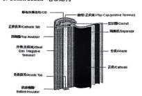
A cell is made of cathode, anode, separator, can and header.
