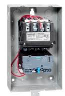
Non-reversing motor starter Size 00 Three phase full voltage Solid-state overload relay OLRelay amp range 3-12A 220-240/440-480VAC 60HZ coil Combination type Indoor general purpose use
