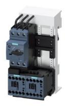
Fuseless motor starter Reversing operation 600VAC Size S00 0.45-0.63A 220/240VAC 50/60HZ screw connection For snapping onto 60 mm busbar systems Type of coordination 2 IQ = 150 KA Also full fills type Of coordination 1 1NC (per contactor)
