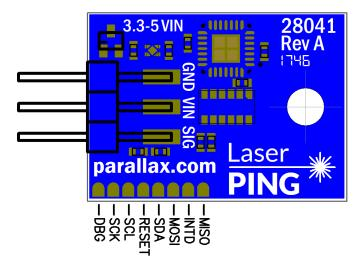
End-user access to the test pads, beyond changing the default mode upon startup from PWM to Serial, is not supported.
