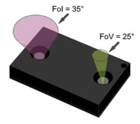
The emitter and receiver elements of the laser sensor form a cone shape. The emitter field of illumination (FoI) is 35°, and the receiver field of vision (FoV) is 25°. The LaserPING sensor will only sense objects within the FoI, but may have reduced sensitivity when bright objects are
