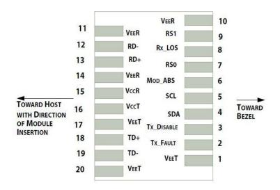
Pin-out of connector Block on Host board
