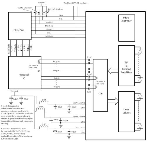
QSFP-DD Optical Module
