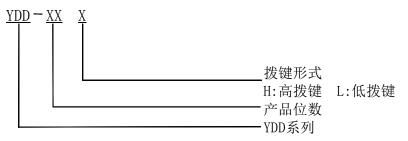
Form of the actuator H:high actuator L:low actuator Position of product YDD Series
