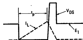
Fig. 2 — Clamped Inductive Waveforms
