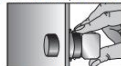
The contact block is snapped on.
