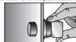
The contact block is snapped on.
