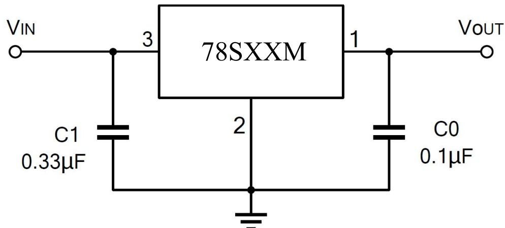
\*Bypass capacitors are recommended for optimum stability and transient response and should be located as close as Possible to the regulators.
