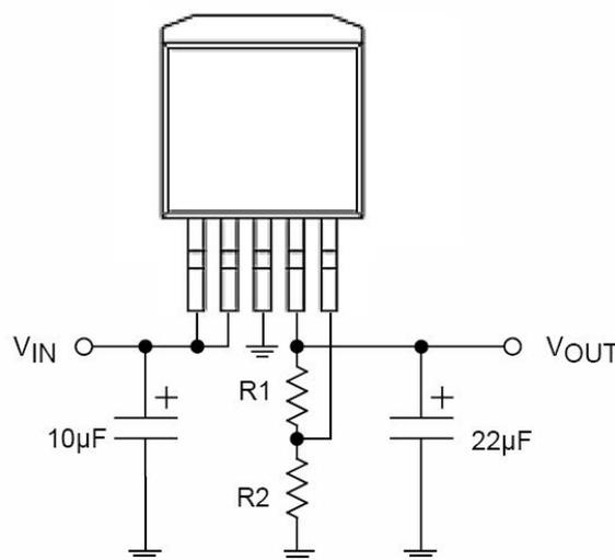
$$V_{OUT} = 1.240V \times \left[ 1 + \left( R1/R2 \right) \right]$$
