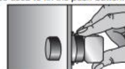
The contact block is snapped on.
