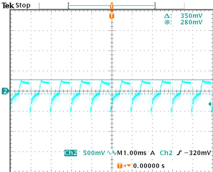
LOAD TRANSIENT WAVE(5V<sub>OUT</sub> 0A~1A)
