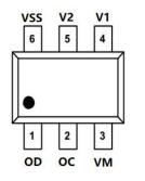
Figure 2. SOT23-6 ( TOP VIEW )
