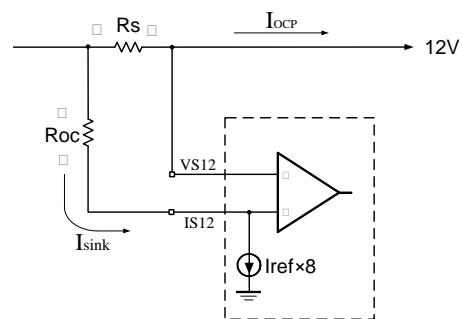
The recommended sense resistor values of RS12A, RS12B, RS5, and RS3 are  $\geq 0.002\Omega$  for good accuracy and enough SNR.
