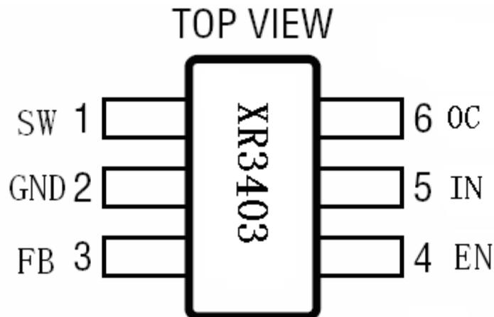
Figure 3. PIN Configuration
