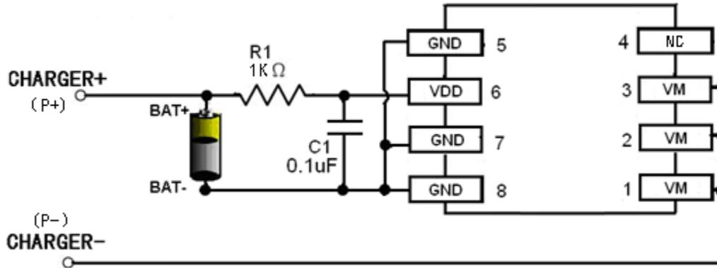
Fig 6 XB8608AJ in a Typical Battery Protection Circuit
