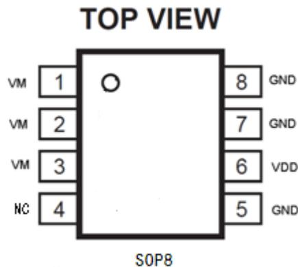
Figure 2. PIN Configuration
