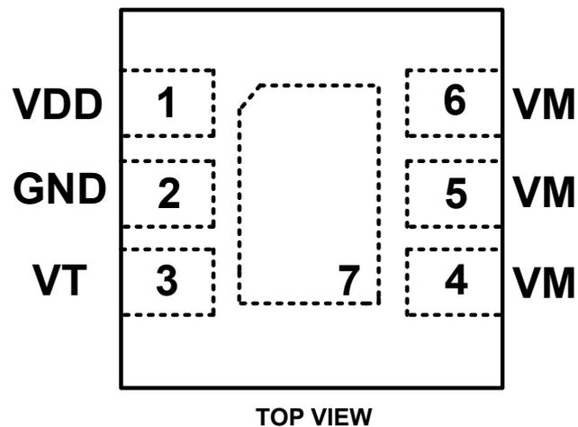
Figure 2. PIN Configuration
