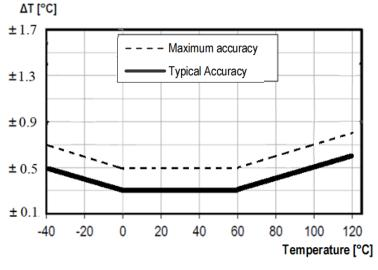
Figure 5. Temperature accuracy of GXHTC3
