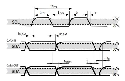
Figure 6. Timing diagram for digital input/output pads.
