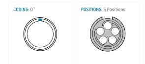
The pin layout corresponds to the view on the termination area
