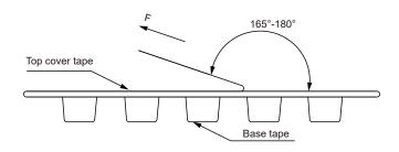
The peel force of top cover tape shall be between 0.15 to 0.78 N
