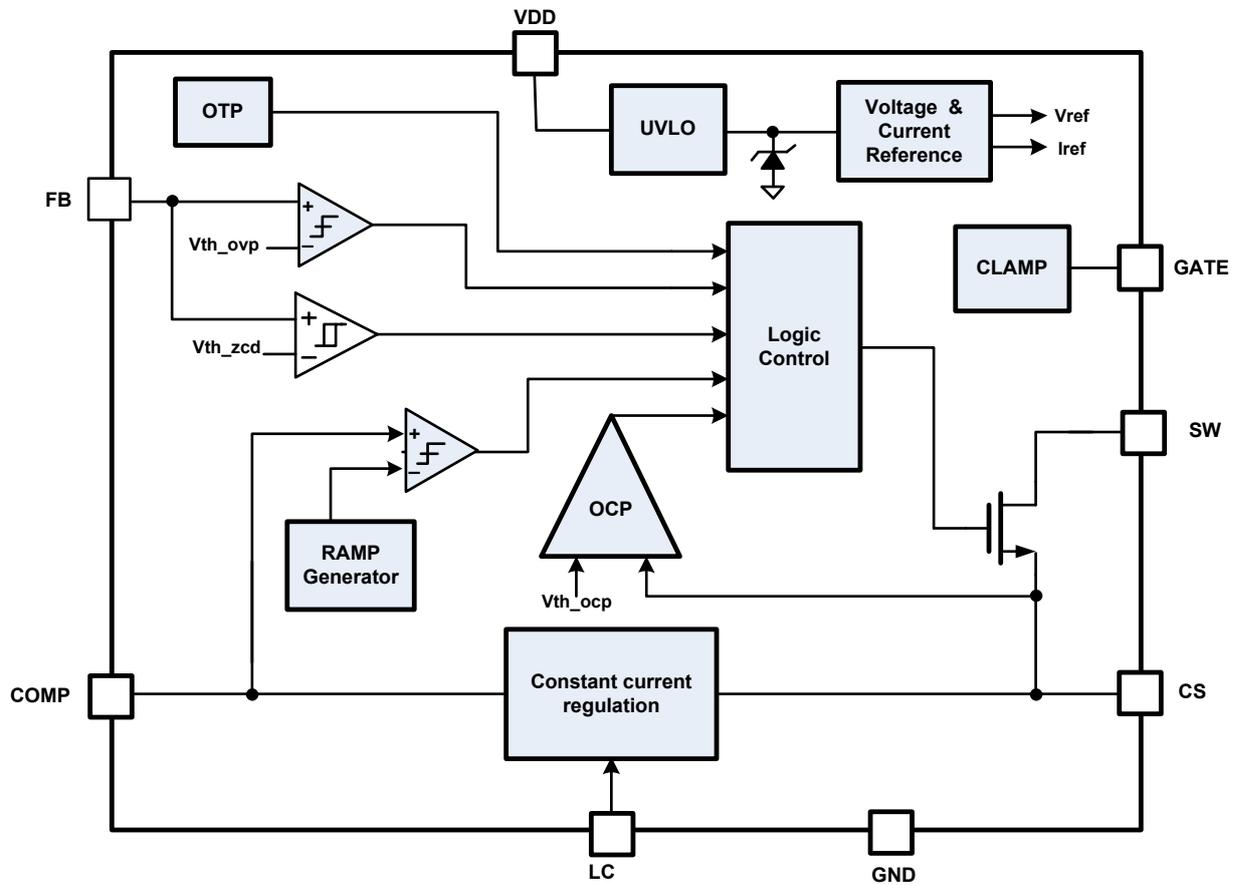
Figure2: OB3638 Functional Block Diagram
