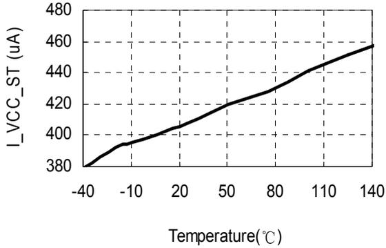
**I<sub>static</sub>(mA) vs Temperature**
