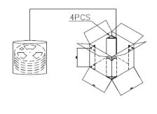
REEL MATERIAL: PET TAP MATERIAL: PET TOLERANCE +/-0.08MM QUANTITY/REEL: 300 PCS
