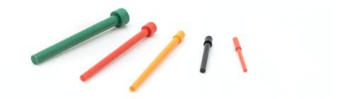
Sealing plugs are used to seal unwired contact cavities. After installing unwired contacts into unused cavities, insert knob end of sealing plug into grommet until it bottoms against the unwired contact per illustration. Install sealing plugs with standard contact insertion / extraction tools.
