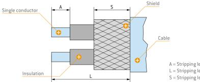
A = Stripping length single conductor L = Stripping length cable jacket S = Stripping length braided shield
