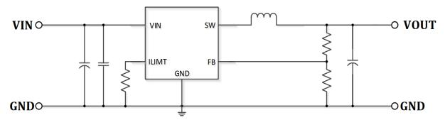
Note: When using a solid or ceramic input Cap, it is recommended to parallel a TVS diode.
