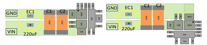
Note: C1, C2 is close to the IC; Pin4, 5 is connected to VIN or GND for easy layout.
