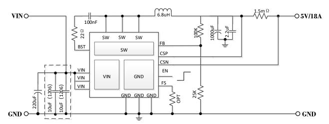
Note: The ceramic capacitors must use two 10uF (1206) or more.
