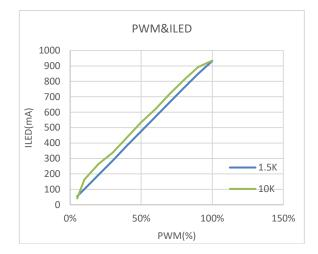
up and pull down, So do not let DIM pin floating.
