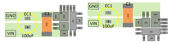
Note: C1 is as close as possible to the IC; Pin4, 5 is connected to VIN or GND for easy layout.
