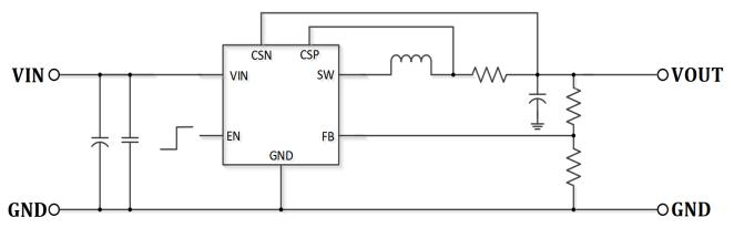
Note: When using a solid or ceramic input Cap, It is recommended to parallel a TVS diode.
