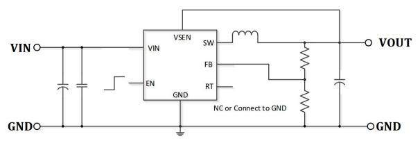
Note: The inductance should be chosen  $\geq$  4.7 $\mu$ H .
