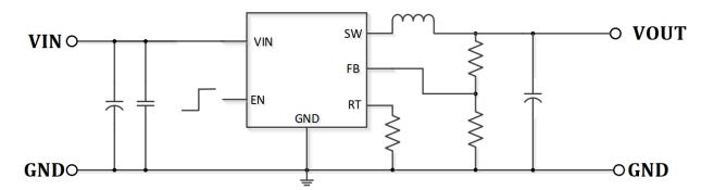
Note: The inductance should be chosen  $\geq 4.7 \text{uH}$ .
