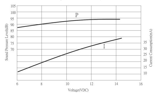
P: Voltage vs. Sound Pressure Level I: Voltage vs. Current Consumption
