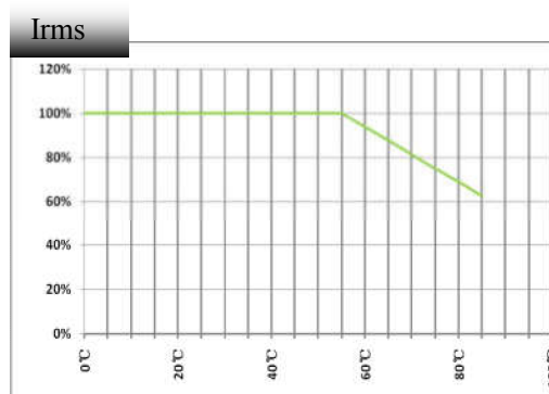
Operating current vs. Temperature
