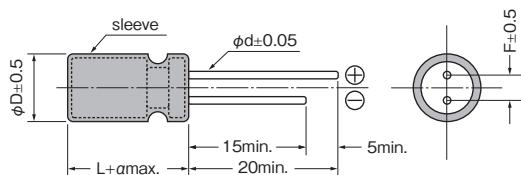
$a : L < 20 \quad a = 1.5, \quad L \geq 20 \quad a = 2.0$ A pressure relief vent is provided for  $\phi D = 6.3$  or bigger
