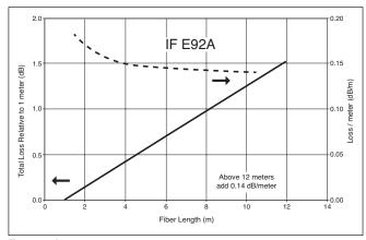
FIGURE 4. Fiber Loss in GH4001
