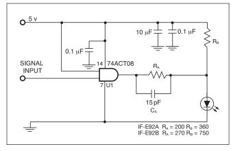
FIGURE 3. Test/Application circuit (IF = 10mA).
