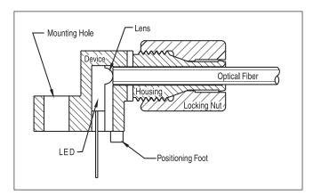
FIGURE 6. Cross-section of fiber optic device.
