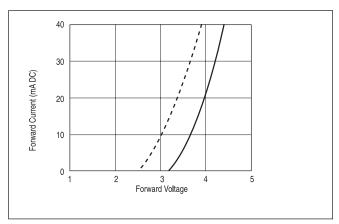
FIGURE 1. Forward current versus forward voltage.
