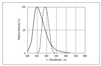
FIGURE 2. Typical spectral output vs. wavelength.
