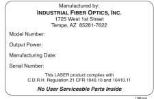
Figure 3. Laser certification and identification label.
