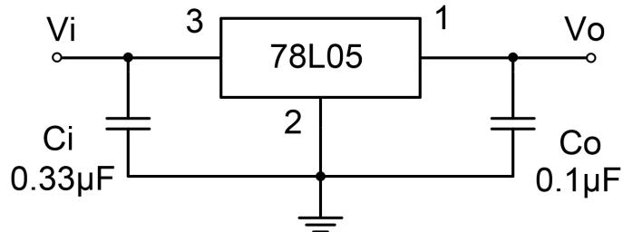
Note: Bypass capacitors are recommended for optimum stability and transient response and should be located as close as Possible to the regulators.
