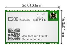
The E200-2G4A20S integrates Microphone and Speaker PA amplifiers internally,
