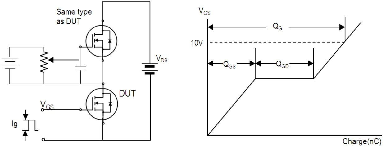
**Fig. 13. Switching time test circuit & waveform**
