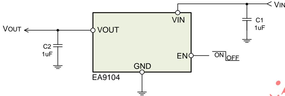
Figure 2. Typical application circuit diagram (Fixed output voltage)
