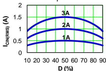
A low ESR capacitor is required to keep the noise minimum. Ceramic capacitors are better, but tantalum or low ESR electrolytic capacitors may also suffice. When using tantalum or electrolytic capacitors, a 0.1 $\mu$ F ceramic capacitor should be placed as close to the IC as possible.
