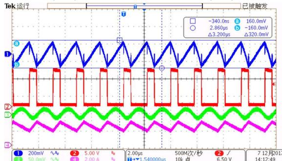
**3. Vout ripple and Switching waveform**
