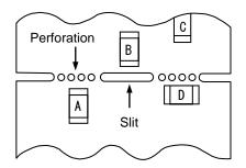
\*1 A > D is valid when stress is added vertically to the perforation as with Hand Separation. If a Cutting Disc is used, stress will be diagonal to the PCB, therefore A > D is invalid.
