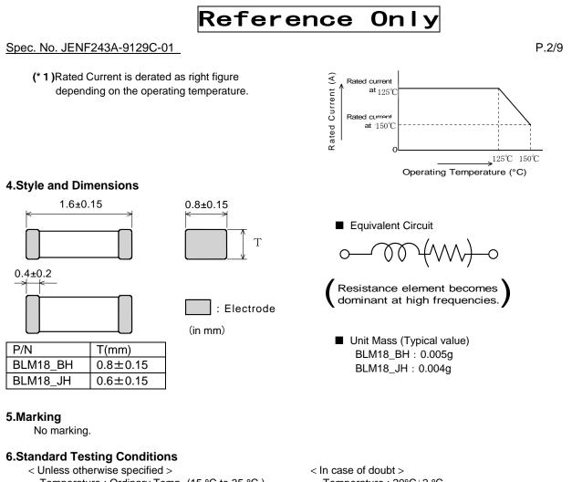
Temperature : Ordinary Temp. (15 °C to 35 °C ) Humidity : Ordinary Humidity (25%(RH) to 85%(RH)) In case of doubt > Temperature : 20°C±2 °C Humidity : 60%(RH) to 70%(RH) Atmospheric pressure : 86kPa to 106kPa
