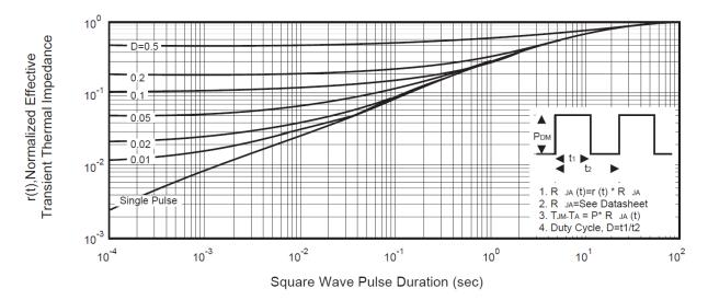
Figure 11. Normalized Thermal Transient Impedance Curve
