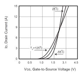
Figure 2. Transfer Characteristics
