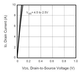
Figure 1. Output Characteristics
