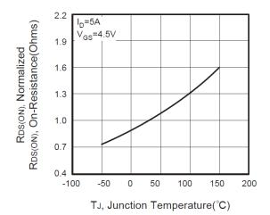
Figure 4. On-Resistance Variation with Temperature
