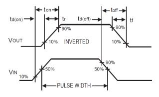
Figure 10. Switching Waveforms
