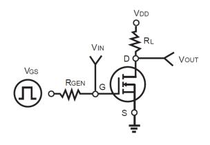
Figure 9. Switching Test Circuit
