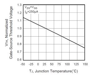
Figure 5. Gate Threshold Variation with Temperature
