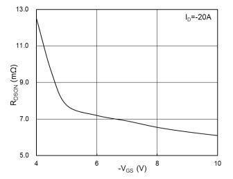
Fig.2 On-Resistance vs G-S Voltage
