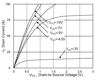
**Fig.1 Typical Output Characteristics**
