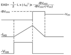
Fig.11 Unclamped Inductive Switching Waveform
