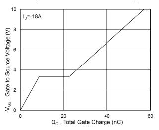
Fig.4 Gate-Charge Characteristics
