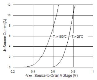
Fig.3 Source Drain Forward Characteristics
