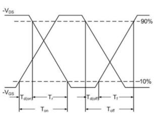
Fig.10 Switching Time Waveform
